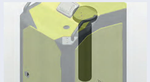
Fig3. Once heated to an optimum 70°C the oil enters a distillation column designed with a dedicated dispersal element.
